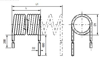
Unextended spiral length Max. extended length of spiral Approx. outer diameter of spiral Approx. outer diameter of spiral
