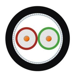
Conductor bare copper wire,
