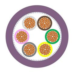
Conductor very fine-wired stranded (32 x 0.1 = 0.25 mm<sup>2</sup> = 24AWG) of bare copper
