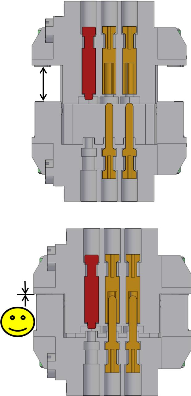
**Pin** in the coded contact chamber on the male side of the connector. A plugging is therefore not possible!
